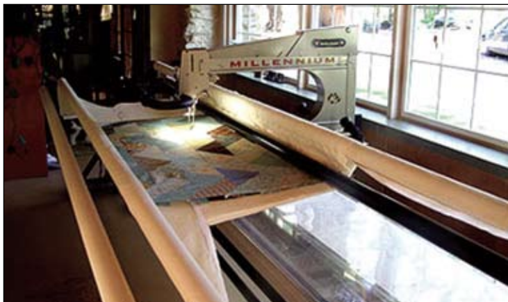
Photo submitted by Patti Middleton A Millennium Long-Arm Quilter at Buena Vista Quilting. The quilter has 14 foot rails and has an on-demand automatic stitch regulator which makes star points and squares.
